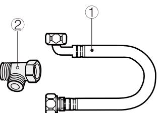
A diagram of the water inlet pipe assembly. It shows a flexible hose (1) with a three-way valve (2) attached to one end.                                                                                                                               |
